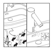
When the LED stays on, cover the sensor window with your hand or with a white card for 20 - 40 seconds to reset the electronics\*.
